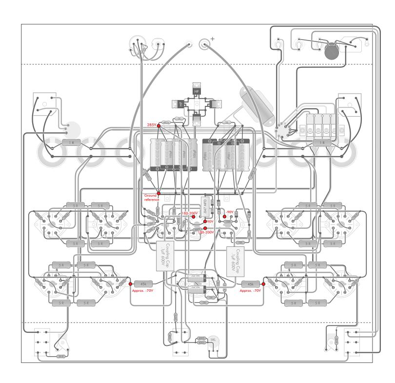
•Test points with voltages; all test points referenced to main ground buss.
