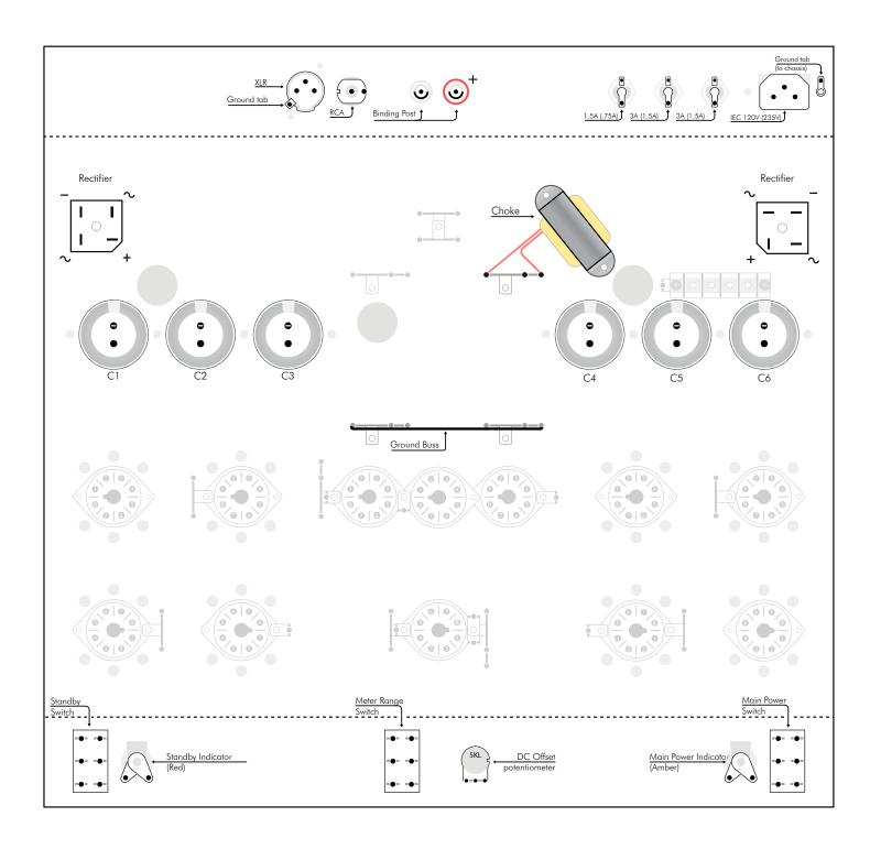
• Notice the orientation of the bridge rectifiers; the positive corners should face the center bottom.
