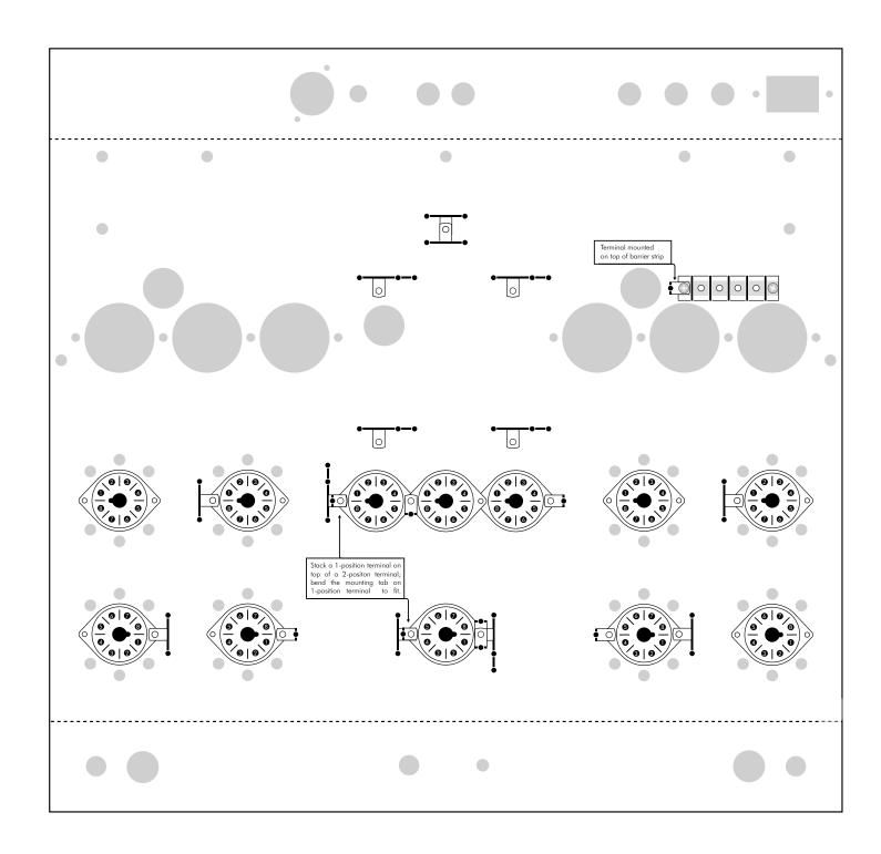
• Note the orientation of the sockets; the key (center hole with slot) in the top row of sockets are all pointed left, and the keys on the bottom are pointed right.
