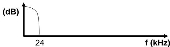
Figure 26. Spectrum After Continuous Time Filter
