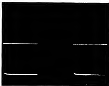
(c) TOP TRACE: GATED OUTPUT 1 \text{V}/\text{DIV} AND 50 \mu\text{sec}/\text{DIV} BOTTOM TRACE: VOLTAGE EXPANSION OF ABOVE SIGNAL—SHOWING NO RESIDUAL 1 \text{mV}/\text{DIV} AND 50 \mu\text{sec}/\text{DIV} —AT LEAST 80 \text{ dB} OF ISOLATION f_q = 100 \text{ kHz}
