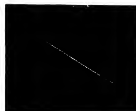
Fig. 8— Oscilloscope photograph of the CA3080 transfer characteristic as applied to the circuit of Fig. 4.
