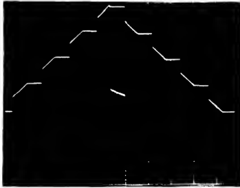
TOP TRACE: SAMPLED SIGNAL 1V/DIV & 20msec/DIV CENTER TRACE: WORSE CASE TILT 20mV/DIV & 20msec/DIV
