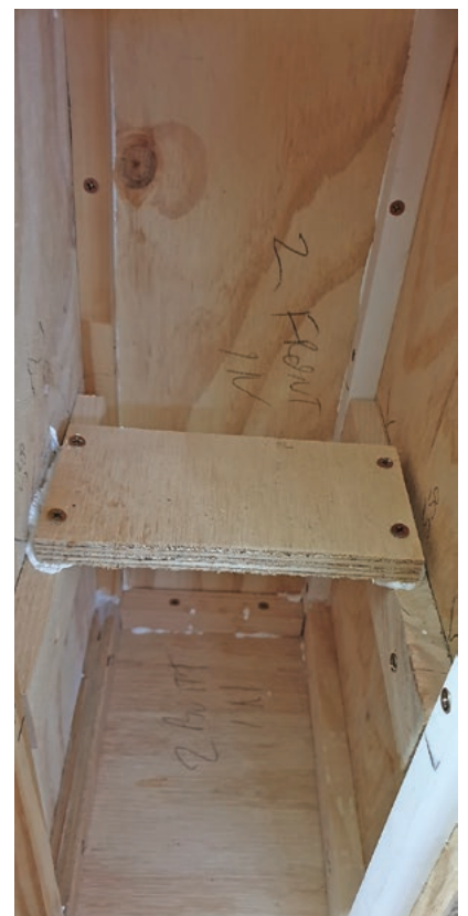
Fig.17: the subwoofer panels are cut from three 600 x 1200mm sheets. As with the monitor speakers, you can cut two of the sheets down the middle. So you don't need to purchase a fourth sheet for just one panel, the last piece is made from one of the bookshelf speaker off-cuts (see Fig.13, last month).
