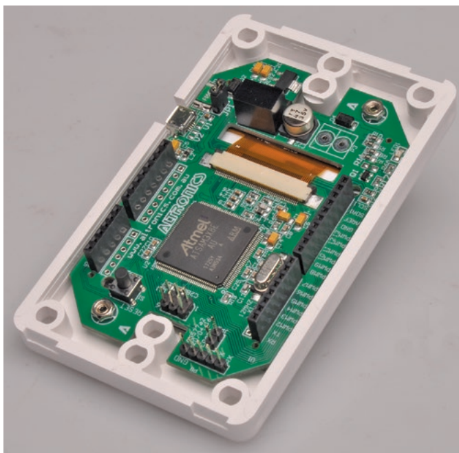
The Altronics K9660 TFT Touchscreen Maker Plate uses the same 32-bit SAM3X8E ARM CPU as used in the Arduino Due to drive a TFT display. It fits in a standard electrical wallplate, changing it from a development platform into practically a finished product.
