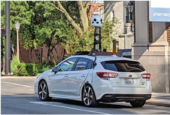
Fig.15: an Apple Maps vehicle near Philadelphia, USA. There are thought to be 12 cameras plus LIDAR sensors in the pod on the roof. Source: David Levy.
