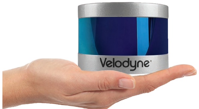
Fig.14: a Velodyne VLP-16 LIDAR device, as used on Google cars.
