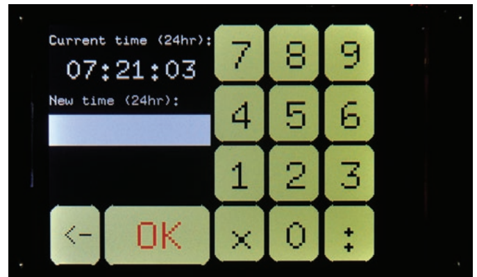
Fig.10: this keypad allows you to update the current time and date as well as set the tariffs and various other tariff-related settings. In this case we're setting the time and pressing OK without entering anything leaves it unchanged. The new time can be entered with or without seconds.
