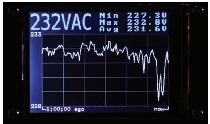
Fig.12: plot of the mains voltage which shows how it varies over a one-hour period. Depending on the location and time of day, the voltage can vary far more dramatically than this. Even so, we can see it varying by more than 1% (2.3V) in a relatively short period of just 30 seconds or so.
