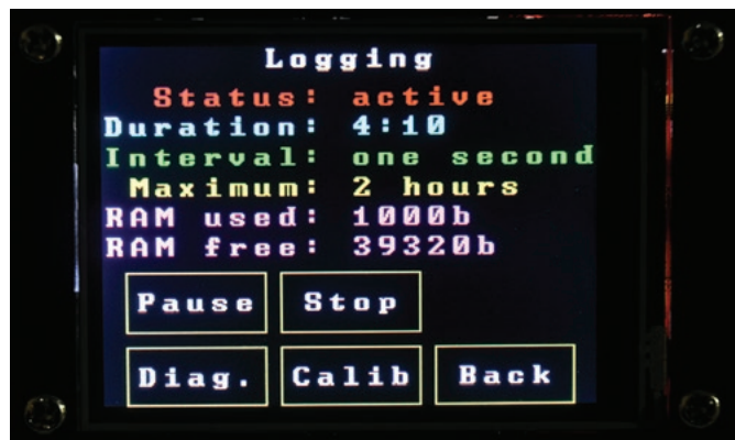
Fig.8: the logging status screen has also been improved since the first article. The same information is shown but there are now buttons to access the diagnostics screen and to perform automatic calibration. The button to dump logged data is not visible because you need to pause logging first.
