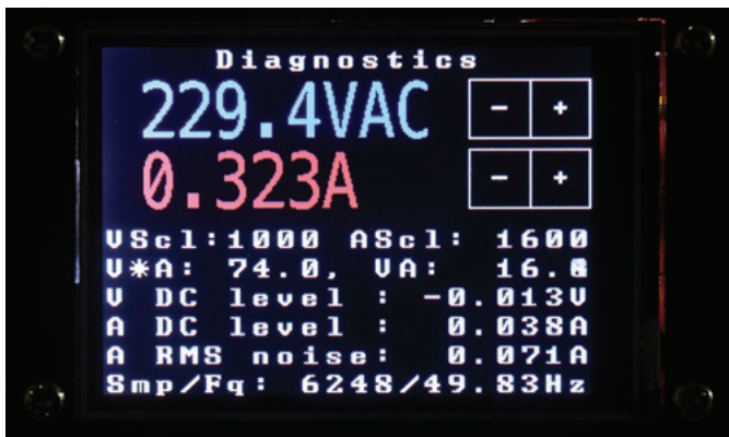
Fig.9: the diagnostic screen which shows the voltage and current readings with extra decimal places and allows fine adjustment of the scaling factors for both. It also displays the automatically calibrated calibration constants below, plus the sampling rate, measured frequency and pre-processing VA figures.
