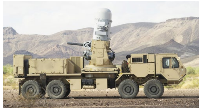
Centurion C-RAM is a land-based version of Phalanx, used for automated base defence against artillery.
