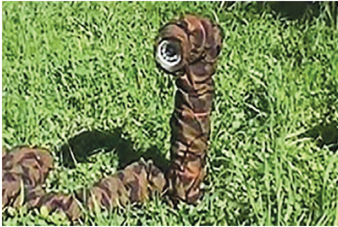
Snake Robot in its natural habitat. Note how the robot has its body raised to get a better view with the head mounted camera.
