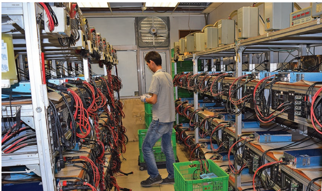
Power supplies on a heat soak cycle at Mean Well. Considering that each power supply is connected to a programmed electronic load, this room must have been using lots of energy, which would place a even bigger load on the air conditioning system. Funnily enough, the English sign above the doorway to this room was "Burning Room". There was no evidence of escaping smoke!
