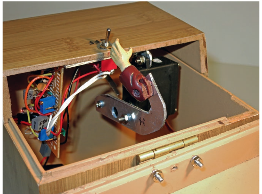
A useless machine is a functional device that serves no useful purpose. This example was designed such that when switched on, a hand will come out and turn the switch off; using a servo to provide the hand with a variable speed.
