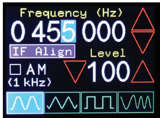
Fig.3: the modified main screen from Geoff Graham's DDS Signal Generator. Note the new "IF Align" button at centre left. You can still use the unit as a signal generator, with all the same functions of the original unit. We simply added the extra functions required for IF alignment, accessed via this new button.
